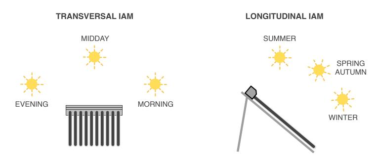
The following table provides the IAM values for Apricus AP Solar Collectors (same for all sizes). A value of 1.00 is when the sun is perpendicular to the collectors surface; so midday for transversal, and mid spring/autumn for longitudinal if the collector is installed at the same angle as the location's latitude.
